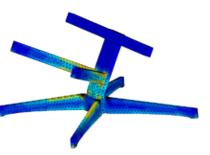
Only a small part of the stand is visible. Inside, multiple internal trusses spread the load over the cabinet. Stress analyses of the stand with FEM (Finite Elements Method) ensures there are no weak areas.
