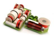
The cross over is paramount to the sound quality. It uses the finest components and is tuned using real time digital filtering techniques, MLS measurements and critical istening.
